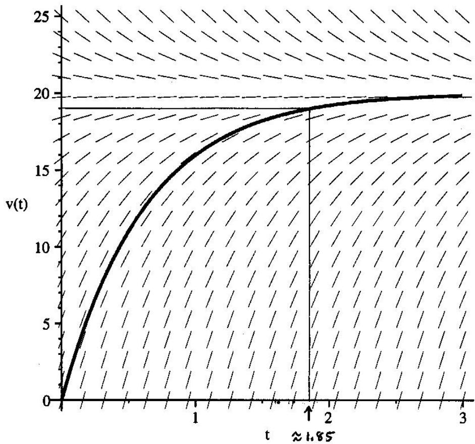
Limiting velocity :  $v_\infty = 20 \text{ ft/s}$
