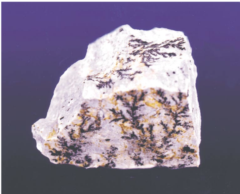
DLA in nature: Magnese oxide patterns on the surface of a rock. (Halsey, Physics Today 2000)
