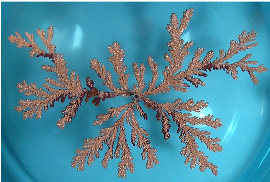
DLA in nature: "A DLA cluster grown from a copper sulfate solution in an electrodeposition cell" (from Wikipedia)
